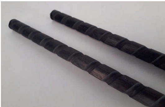
Figure 4: Carbon reinforcement bar | photo: Schulze-Ardey
