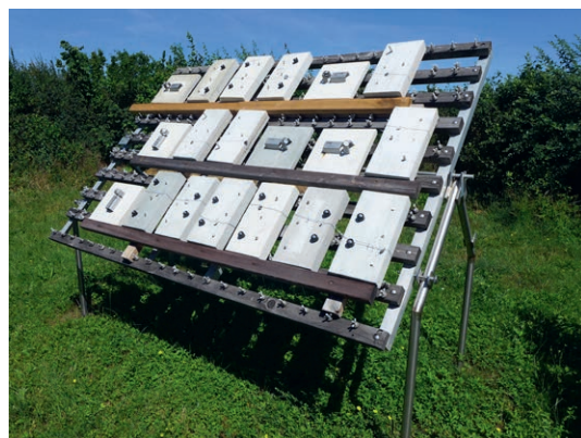
Figure 7: Carbon concrete slabs with built-in parts on the free weathering stand of the Institute for Corrosion Protection in Dresden | photo: Jürgen Triebert
