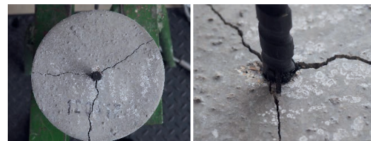
Figure 7: Splitting failure at UHPC | photos: Frank Schladitz
