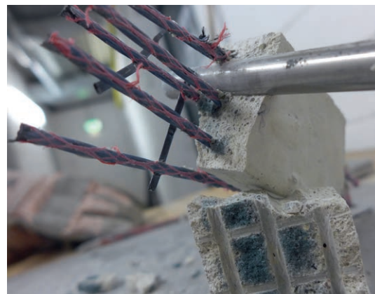
Figure 9: Opened test specimen of one variant N (B2 Hf modified and CO 2 ) after exposure in the climatic chamber: no corrosion between carbon fibre grid and stainless steel insert | photo: Jürgen Triebert
