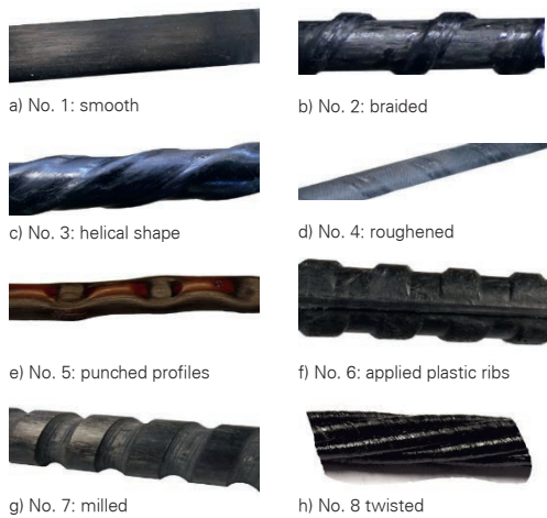
Figure 1: Used carbon rebars | graphic: Alexander Schumann
